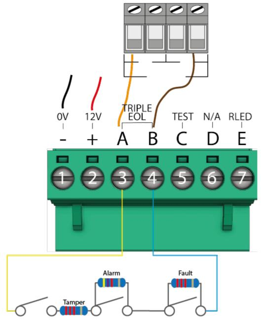
Fault Monitoring - A fault will be indicated by one of the following:
