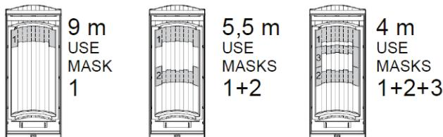
Masking using strips of the supplied foil can also be used to avoid unwanted moving objects (e.g. a tree). Use the supplied protective hood for protection against the sun and rain.
