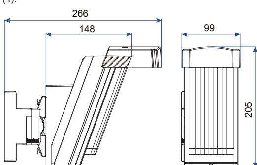
Figure 5: Detector dimensions
