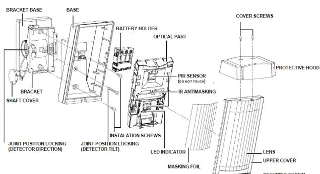
Figure 3 detector configuration
