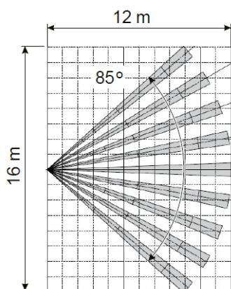
The above-mentioned detection characteristics apply if the detector is installed vertically in the guarded area. If a shorter detection range is required, do not tilt the detector on the joint. Use the supplied self-adhesive mask foils:
