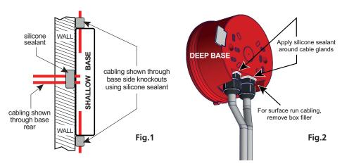
\* For IP65C rated models, carefully remove the factory fitted IP55C O ring from the deep base and carefully fit the supplied IP65C O ring (Pt. No. RNU0100054). It is important to use a plentiful amount of silicone based lubrication on the O ring to assist fitting the sounder to its base.
